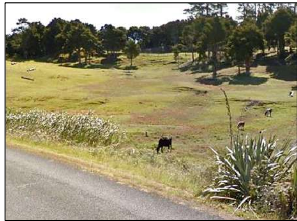
Photo 10: Hummocky ground and evidence of shallow soil creep in Undifferentiated Mangakahia Complex in the northwest of the site.
